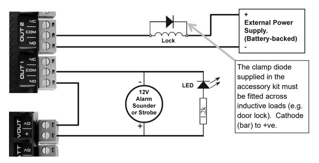
**Lock or Solenoid Control.** An External Power Supply is recommended to power inductive loads to protect the controller, provide longer battery backup & minimise the possibility of earth loops.
