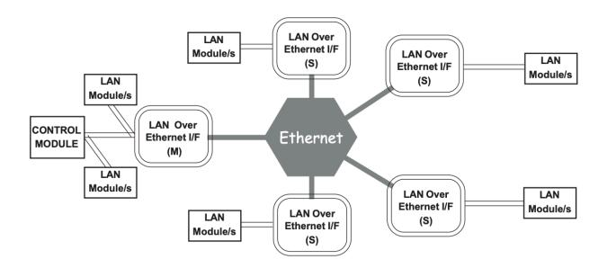
LAN Over Ethernet interfaces cannot be used in a "daisy-chain" configuration
