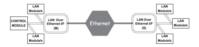
Up to 4 Slave units can be connected to the Ethernet network to connect the Control Module RS485 LAN to one or more other Modules in a number of remote locations.
